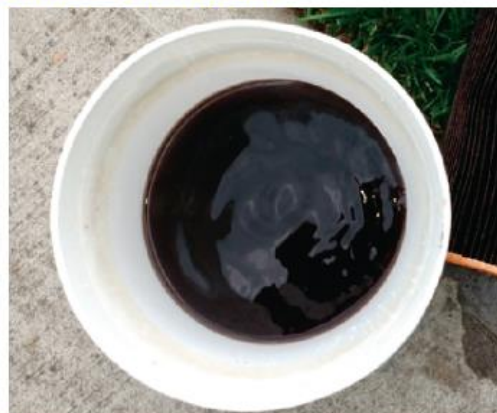
Figure 2. Mn-oxides causing black water in an AQUA-NC supply
