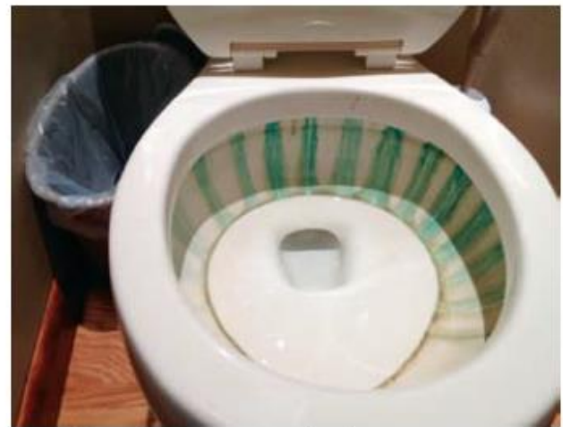
Figure 1. Blue-green stains in a toilet due to copper corrosion by acidic water.
